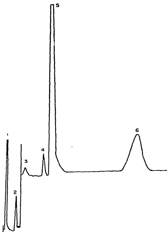
Fig. 6. Chromatogram of hydrocarbon mixture illustrating class separations. Peaks: 1 = hexane; 2 = decane; 3 = water; 4 = propionaldehyde; 5 = acetone + methanol; 6 = benzene.
